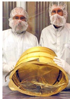
Fig. 8. Concentrator as recovered in Utah. Interior portions of this structure experienced effects of focusing voltage. [18]
