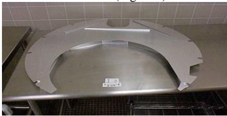
Fig. 4. Canister thermal shield prior to installation. Diameter is 75 cm.
